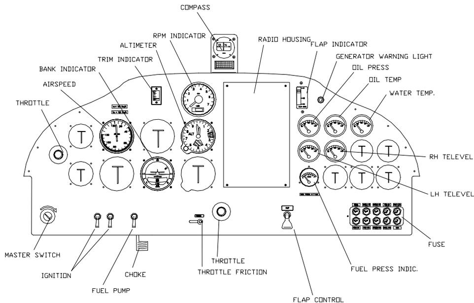
Figure 1-2 Instrument Panel
